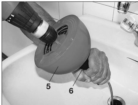
**Make sure that the drill is disconnected from the hexagonal adaptor when the cleaning coil is being pulled back into the housing.**
