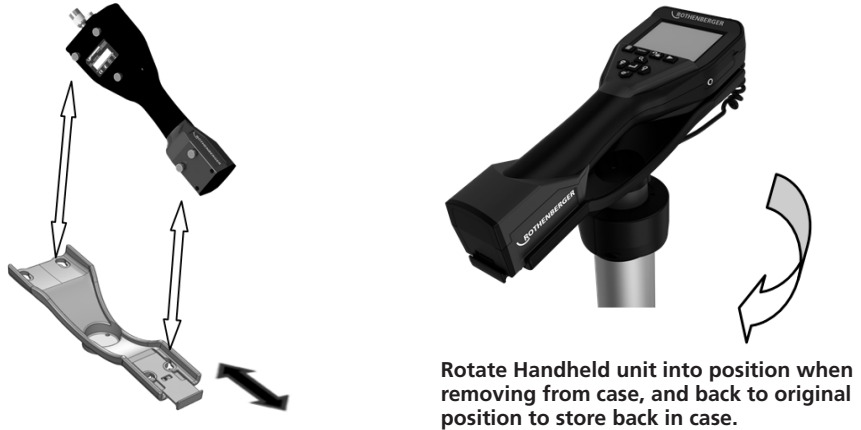
Figure 4 – Installing ROSCOPE 1000/i2000 handheld unit to the mounting cradle
